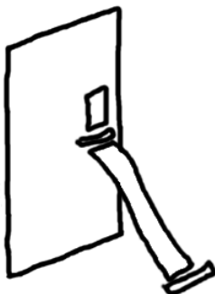
Figure 4.1: Using bracing to secure a door
